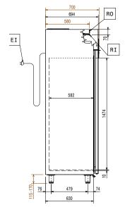
Electrical inlet (power) ΕI Refrigerant Inlet RΩ Refrigerant Outlet
